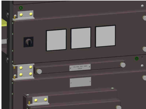
Upper test point access
