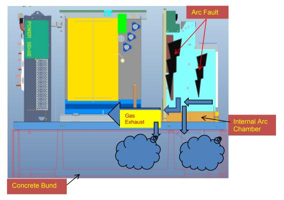
Figure 4 – Arc Chamber (gas flow)
