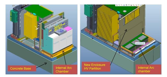
Figure 1 – Arc Chamber (enclosed)
