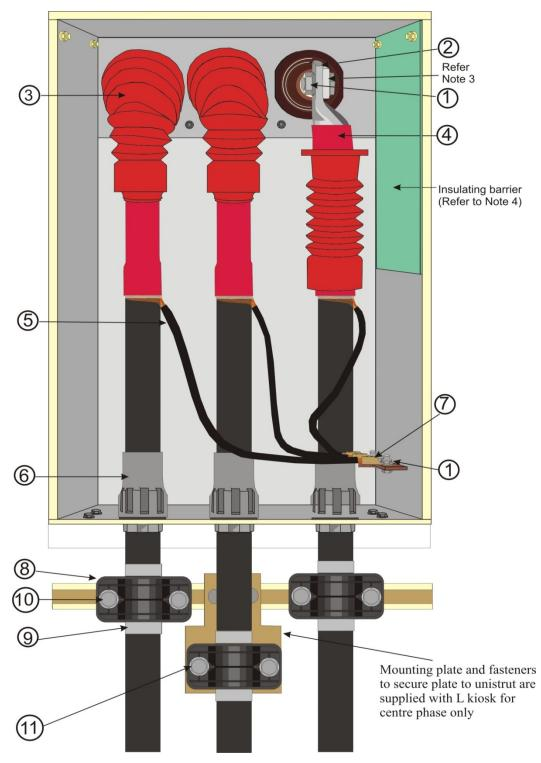
Figure 10-14 – Indoor Termination into Non Arc Chamber RM6 Switchgear (Left hand side feeder endbox shown)
