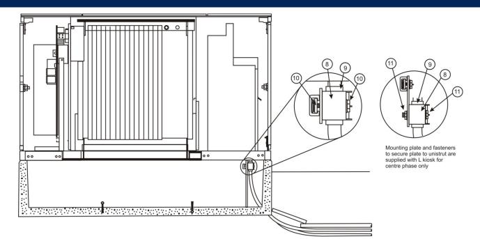
Figure 10-15 – Cable Clamping Details (side view)
