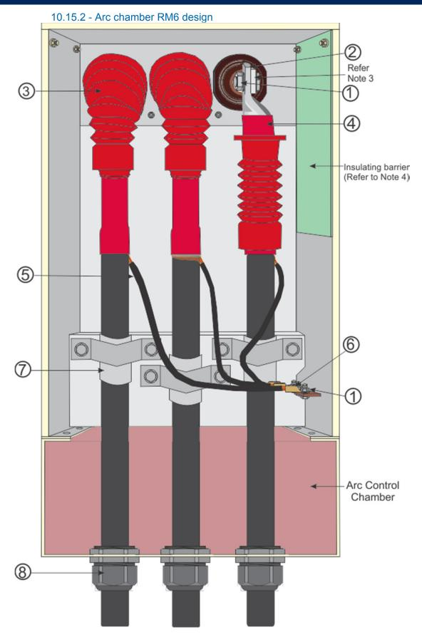
Figure 10-15A – Indoor Termination into Arc Chamber RM6 Switchgear (Left hand side feeder endbox shown)
