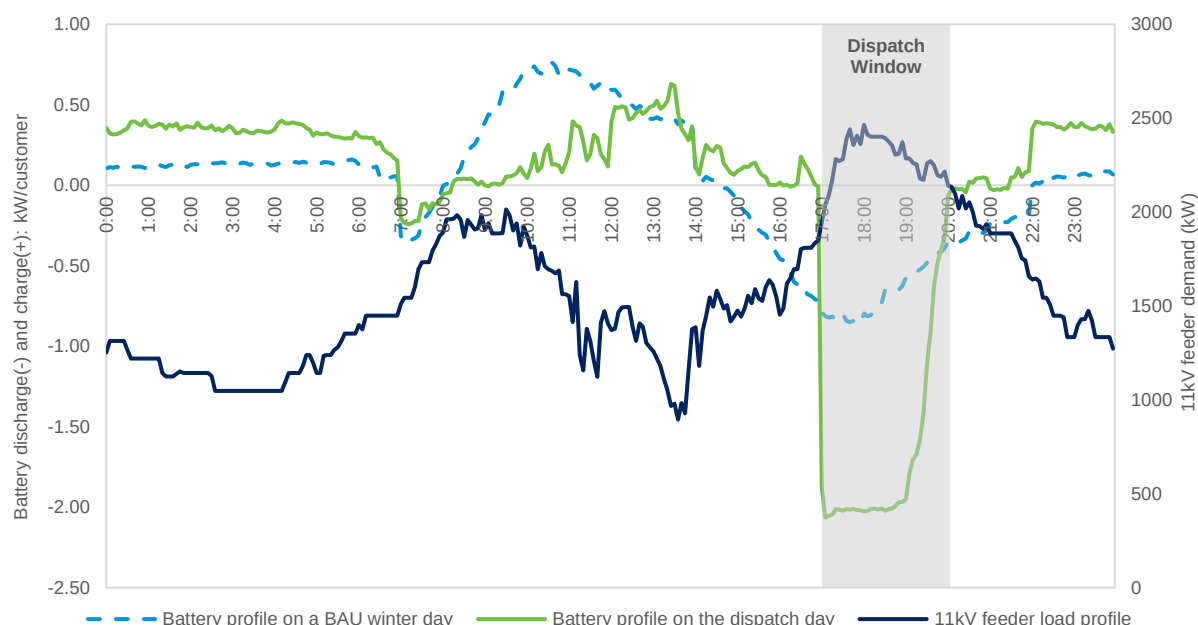
Figure 4.7: VPP profile compared against load profile of 11kV feeder 80923 at Kurri zone on 14 July 2020
