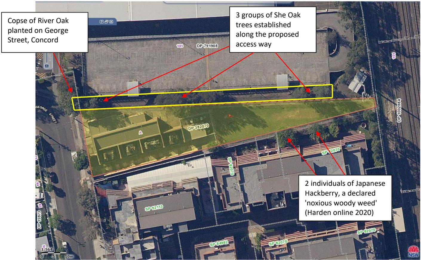
**Figure 1** - The location of the Concord Zone Substation (bounded in red) and indicative access path of about 100m in length from George Street, Concord, where 3 groups of She Oak trees are proposed for removal to allow access for heavy vehicular traffic (bounded by yellow font)
