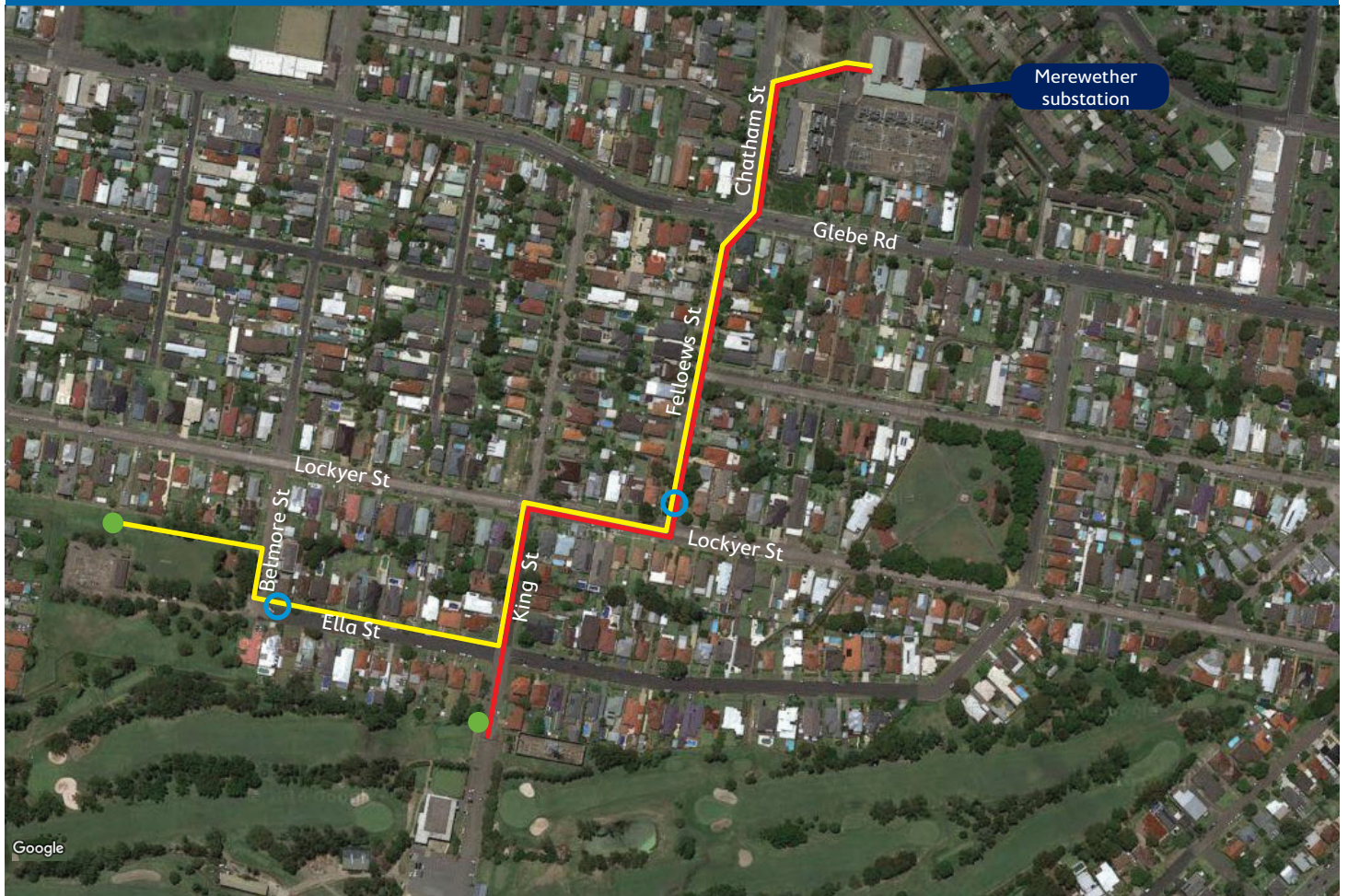
— Feeder 766 route — Feeder 760 route ○ Joint Bay/Pulling Pit ● New UGOH locations are indicative
