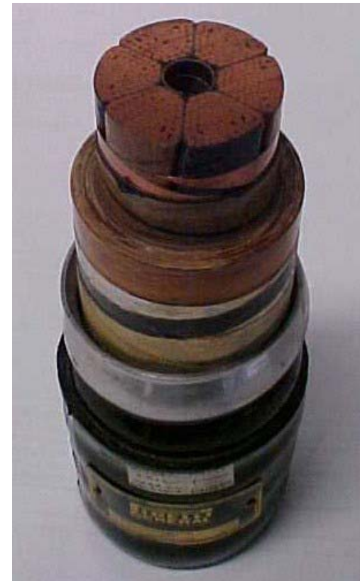
132kV cable cross section
