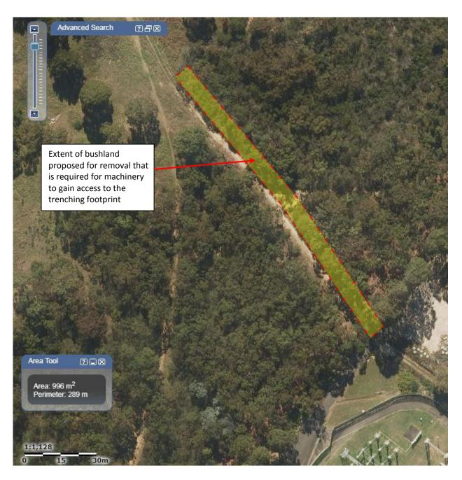
**Figure 2** – Proposed area of bushland required to be removed/trimmed for trenching works at Georges River National Park, Revesby Heights, to install the new 132kV line to the substation shown at the south-east section of the image (sourced from SIXmaps OEH 2018).
