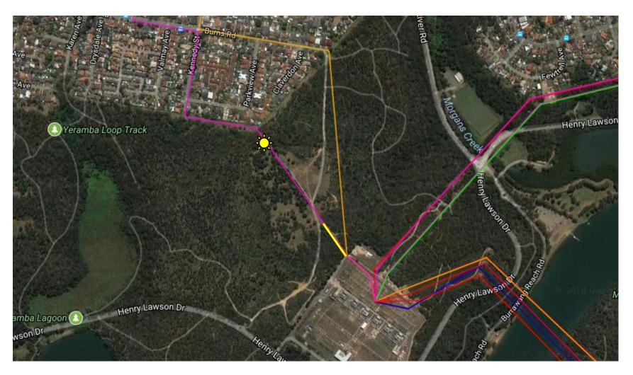
**Figure 1** - Aerial image of subject area indicating the proposed route of the feeder from Kennedy Street, Revesby Heights, to the Sydney South Substation (marked in purple outline) requiring some trenching through bushland (bold yellow outline) for the works to occur
