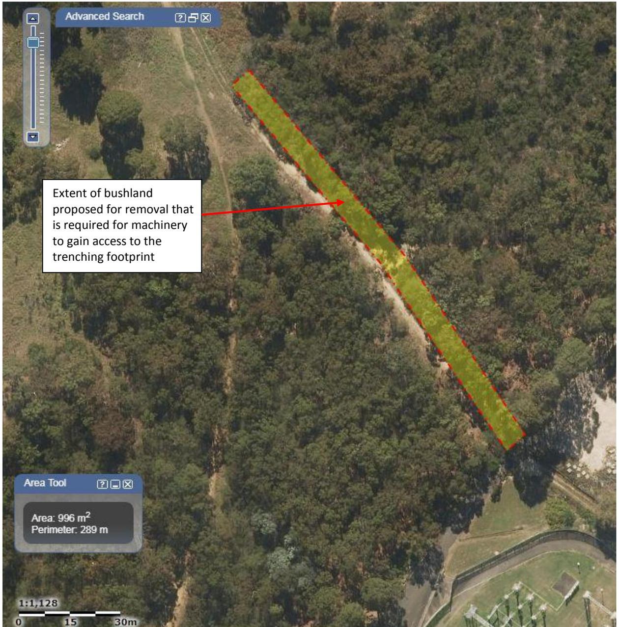
**Figure 2** – Proposed area of bushland required to be removed/trimmed for trenching works at Georges River National Park, Revesby Heights, to install the new 132kV line to the substation shown at the south-east section of the image (sourced from SIXmaps OEH 2018).
