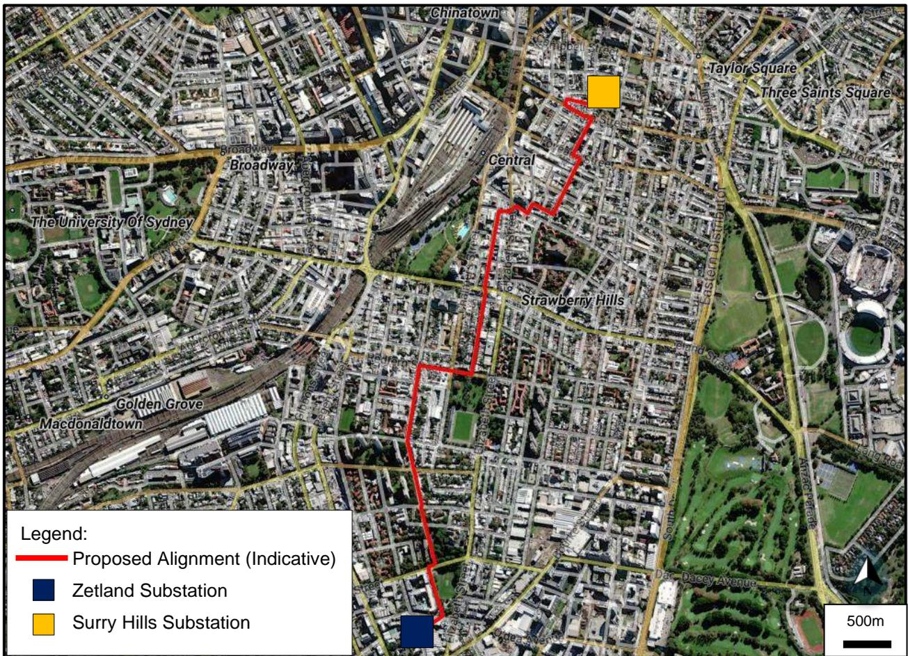
**Figure 1 - The Alignment Location & Aerial Image (extracted from MinView)**
