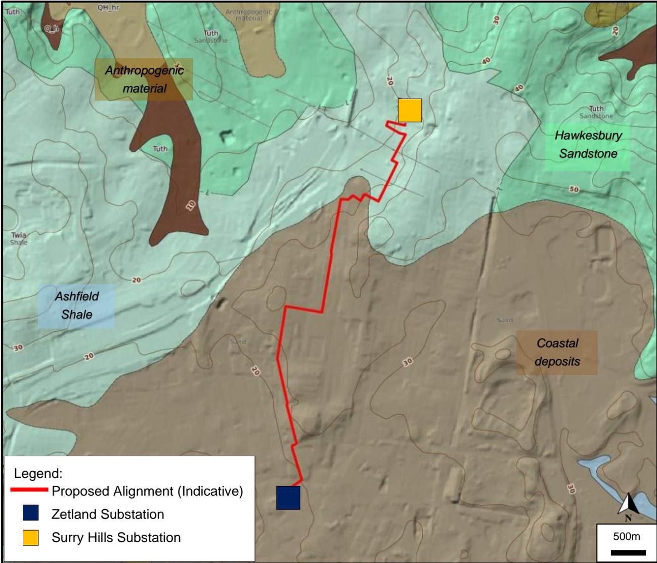
Figure 2 - The M2SH Alignment with NSW Seamless Geology and 10m Contours
