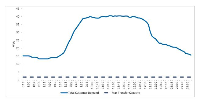
Figure 6 – Summer maximum demand profile at City East zone substation with maximum load transfer
