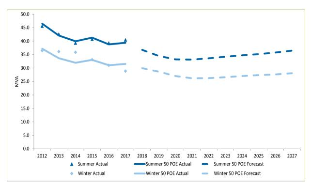
Figure 1 – Demand forecast at City East zone substation
