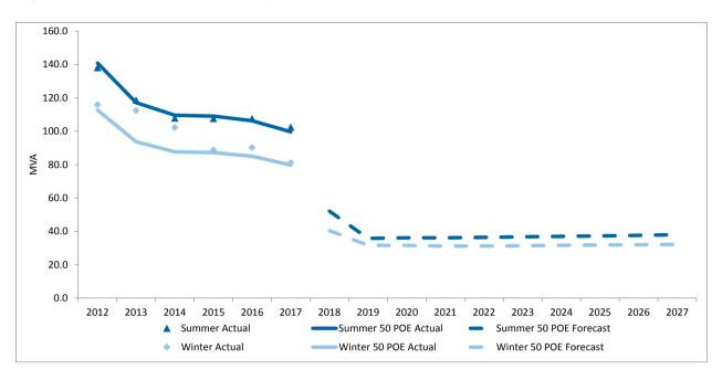
Figure 2 – Demand forecast at Dalley Street zone substation
