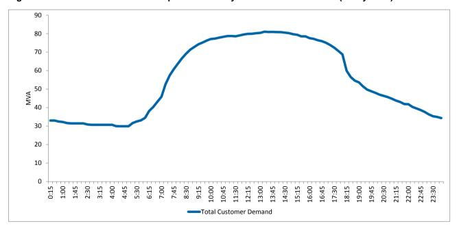
Figure 9 – Winter maximum demand profile at Dalley Street zone substation (4 May 2016)
