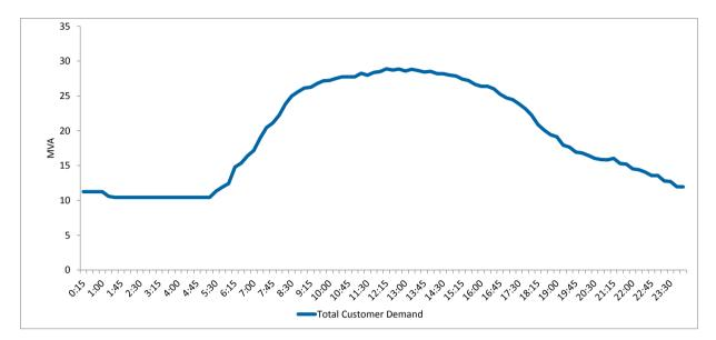
Figure 4 – Winter maximum demand profile at City East zone substation (23 May 2016)
