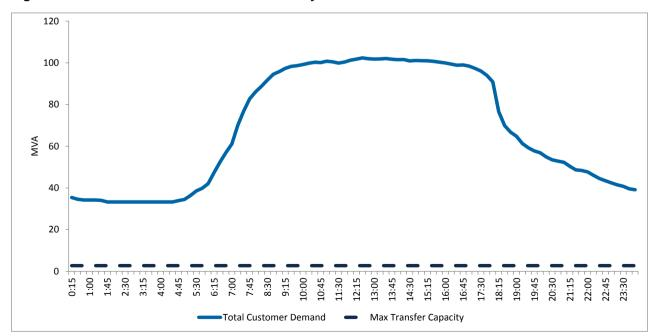
Figure 11 – Summer maximum demand at Dalley Street zone substation with maximum load transfer
