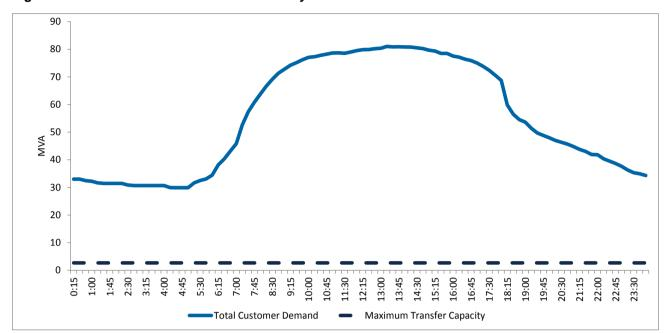
Figure 12 – Winter maximum demand at Dalley Street zone substation with maximum load transfer
