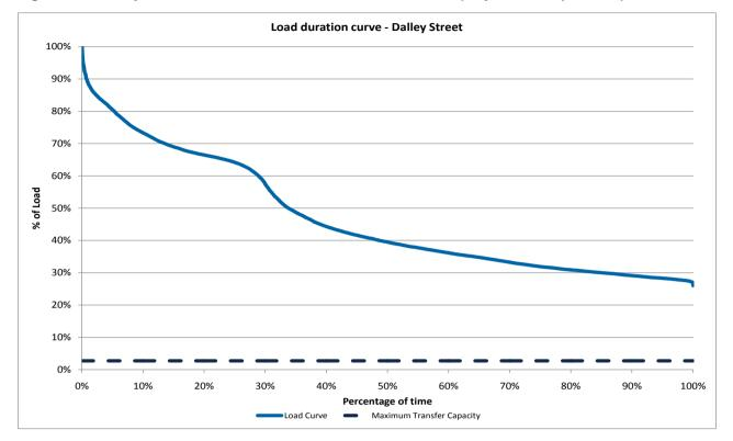
Figure 10 – Dalley Street Zone Substation Load Duration Curve (May 2016 to April 2017)
