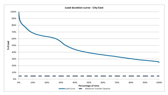
In the event of a network outage on a maximum summer peak demand day, after use of the maximum transfer capacity in an emergency switching of the network, there is a shortfall of network supply from 0:00 to 24:00 or 24 hours. The maximum shortfall in network supply on 30 January 2017 would have been 38.7 MVA at peak and 11.5 MVA at off peak times (overnight). See Figure 6 below.
