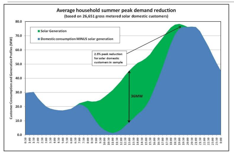
Total solar panel capacity of domestic customers in sample around 52 MW.
