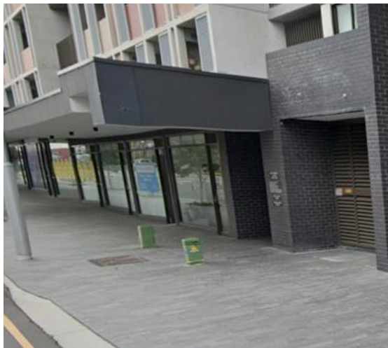
Fig B21 - Unacceptable – the pillars are adjacent to the property boundary, but the building setback means they are in the middle of the footpath.
