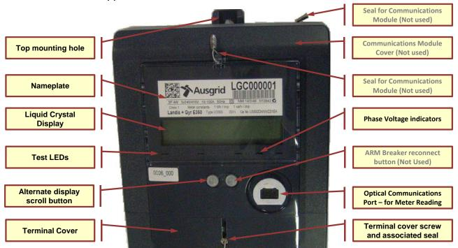
Figure 5.4-3: LGC Meter layout
