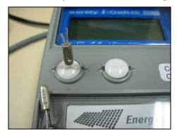
Figure 4.2-8 Sealing the Left button
