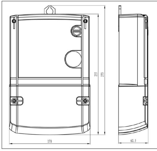
Figure 3.2-2 HLE Meter dimensions
