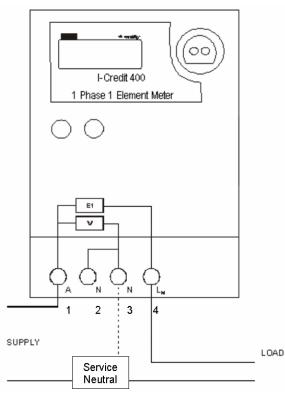
Figure 4.2-4 i-Credit 400 meter wiring schematic
