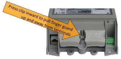
The finger guard must be reinstated after conductors are securely terminated
