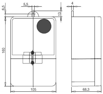
Figure 8.2-3 Ripple Receiver Dimensions
