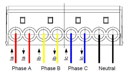
Figure 6.1-7: EET Mains Connection diagram
