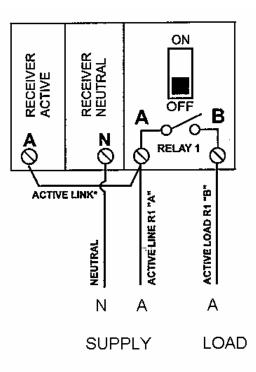
Figure 8.1-3 details the wiring schematic diagram for the relay.
