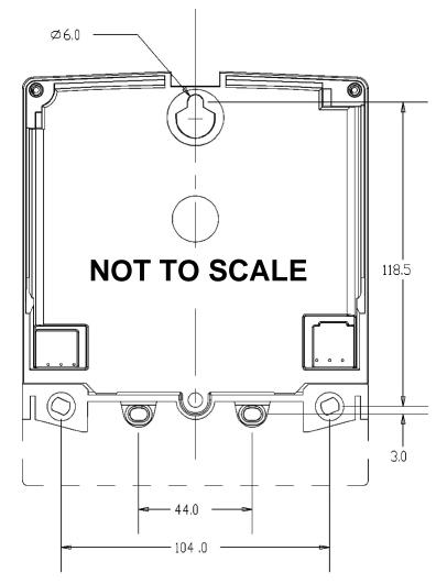
Figure 4.3-2: EEL Mounting Diagram
