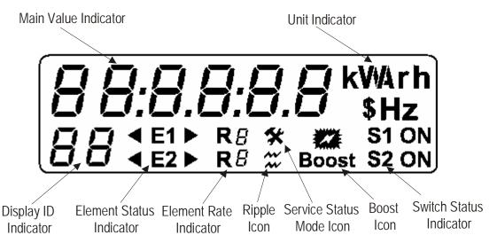
Figure 5.1-2 i-Credit 400 meter display (Note the Boost feature is not used by Ausgrid)
