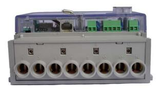
Figure 6.1-5: EET meter terminals
