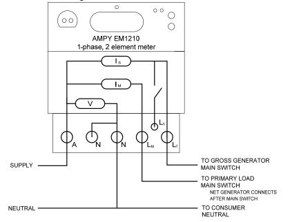
Figure 5.2-8 Wiring Schematic for Gross + Net Spacesaver – Structure 29
