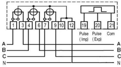
Figure 3.2-4 HLE meter wiring schematic
