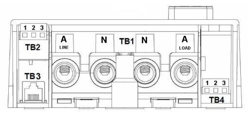
Figure 4.3-6: EEL terminal block diagram
