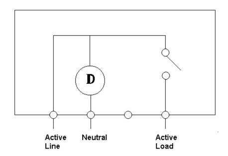
Figure 8.3-2 Bottom connect terminal arrangement
