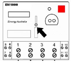
Figure 4.1-6 EM1000 meter seal location
