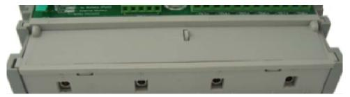
Figure 5.5-5: ECP Terminal Finger Guard
