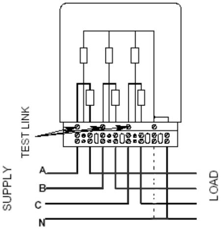
Figure 3.1-5 AMT meter wiring schematic
