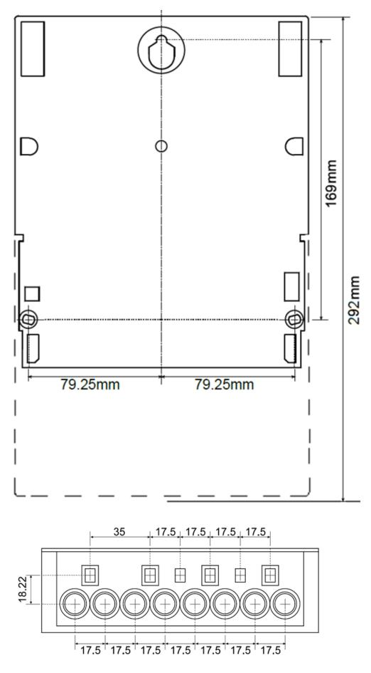
Figure 5.5-1: ECP meter dimensions (not to scale).
