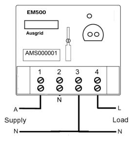
Figure 2.1-4 EM500 meter wiring schematic
