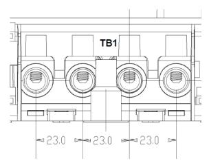
Figure 4.3-3: EEL Main Terminal Spacing
