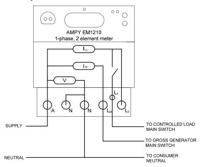
Figure 5.2-7 Wiring Schematic for Gross Metering – Structure 27
