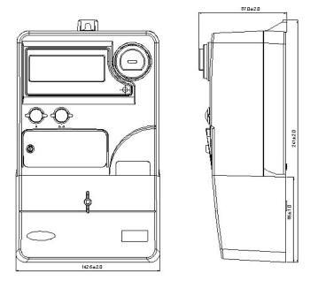
Figure 4.2-3 Meter Dimensions
