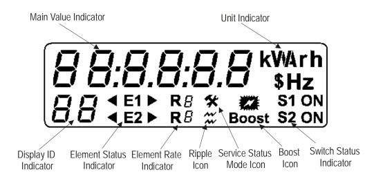
Figure 4.2-6 i-Credit 400 meter display
