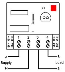
Figure 4.1-4 E1000 meter wiring schematic
