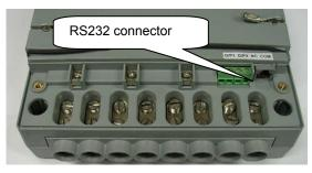
Figure 6.2-6 Terminals and RS232 connector
