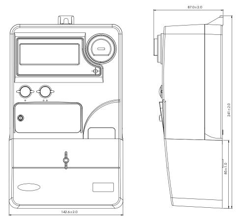
Figure 5.1-4 Meter dimensions and mounting diagram
