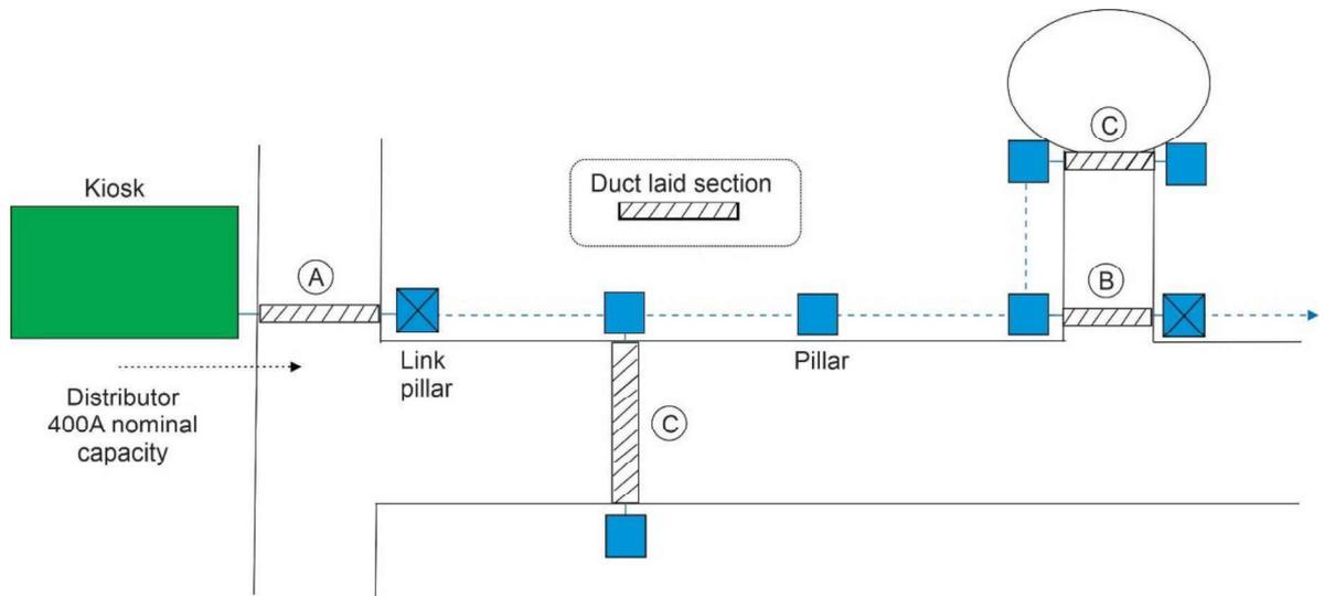
A & B : Duct laid sections forming the main distributor loop require a 400A rating. (Min 300AL)
