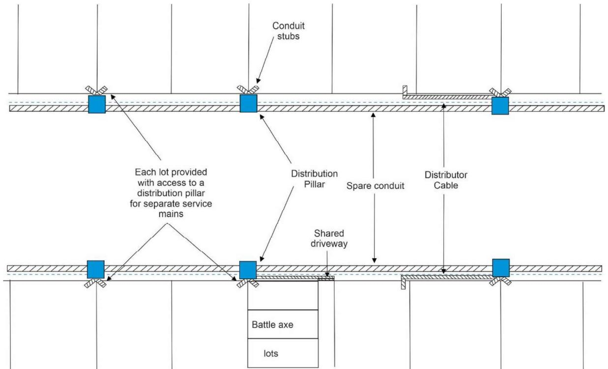
C3 Duct laid sections of low voltage distributor
