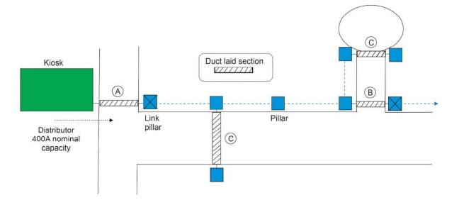
A & B : Duct laid sections forming the main distributor loop require a 400A rating. (Min 300AL) C: Duct laid sections that supply a maximum 15 services with no alternate supply may utilise 240AL.
