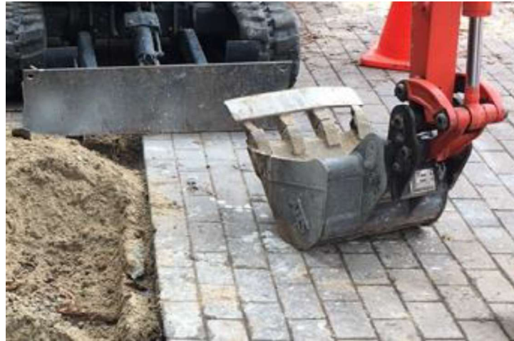
Figure 2: Example of excavator bucket without exposed teeth.
