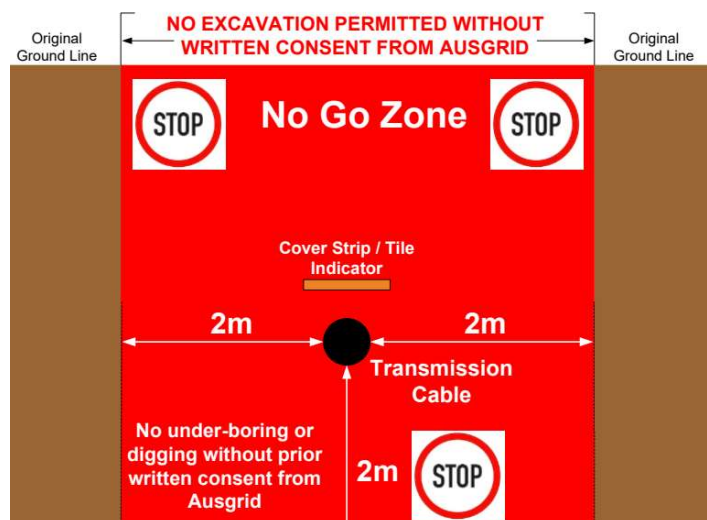
Figure 3: Requirements when excavating near Transmission cables.
