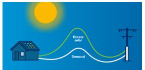
On sunny days, rooftop panels can generate more electricity than homes are using, and the grid can struggle to absorb the extra energy. This can lead to clean energy going to waste, voltage problems, and limits on how much solar power people can export.
