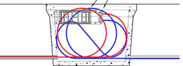
TYPICAL CABLE FLOW FOR FIBRE CABLE WHERE CABLE ENTERS PIT FROM EITHER END \* WITH SPLICE CLOSURE \*
